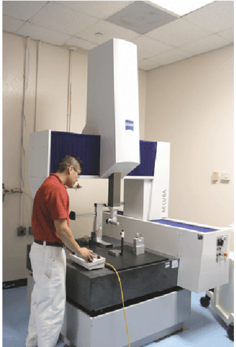
Victor Ruiz, receiving inspector-CMM operator, sets up a part for inspection on the new Zeiss Accura CMM.
